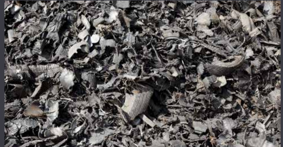
Shredded waste tyres, when mixed with chemical wastes, wood or coal, can be burned in power plants, paper mills and concrete kilns.
