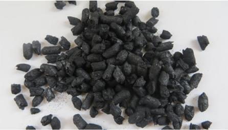
A thermal conversion process known as pyrolysis, which heats biomass in a reactor vessel containing an oxygen-free atmosphere, can be used to reprocess tree cuttings and other woody material into a solid product known as biochar.
