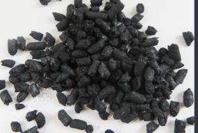
Biochar is created by transforming organic material such as wood waste through a thermal process known as 'pyrolysis'. This valuable bioproduct offers a wide variety of benefits including carbon capture, water treatment, odour control, industrial applications and soil improvement.
